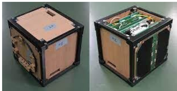
Image n°16 : Prototype du satellite Lignosat © KOJI MURATA / KYOTO UNIVERSITY
